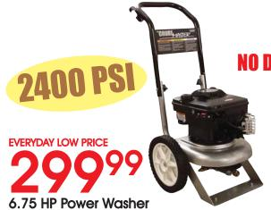
2.0 GPM. 2400 PSI. AR triplex pump, aluminum manifold, thermal relief valve, 25' hose, insulated pro style gun, 1/4" steel wand, 0-60° adjustable nozzle, detergent inject feature, 12" semi-pneumatic tires, 1-1/4" steel tubing frame, rubber isolators. 1 yr. limited warranty. #1023258.
